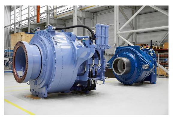
Technological leap made visible: thanks to the increase in power density, wind gearboxes are now more powerful and at the same time more compact than 10 years ago. An older 6-megawatt gearbox at the front and the much more compact new 7.2-megawatt gearbox at the rear.
